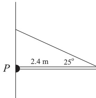
Figure 5: The rope is attached to the wall at one end and the rod at the other.  $P$  is the pivot.
