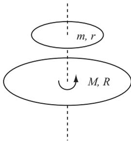
Figure 2: The upper disk, initially at rest, falls with negligible speed on the lower one which is spinning. Their centers coincide.
