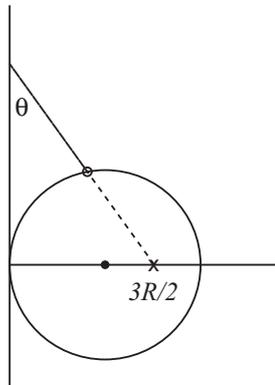
Figure 4: The rope is attached to the wall at one end and the ball at the other. If extrapolated, the line of the rope crosses the horizontal line going through the center at a distance  $3R/2$  from the wall.
