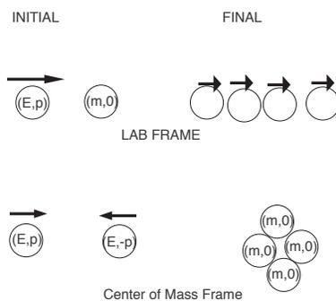
Figure 3: The reaction seen in lab and CM frames. ( $E$ =Energy,  $p$ =momentum) given in brackets. Arrows indicate the spatial motion.
