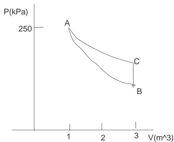
FIG. 1. The segment AB is adiabatic and CA is isothermal despite my rendering.
